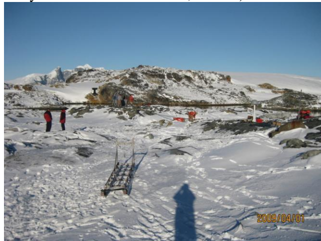
Figure 3: Photograph looking approximately southeast toward the GPS receiver (right) and the power array (left). Note that the connecting cable between the two was bridged with iron pipe to avoid ice hazards in the small melt pond.
